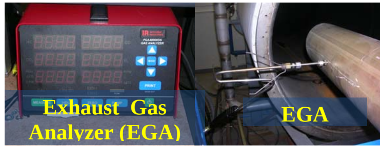
Figure 14 Exhaust Gas Analyzer and its Probe
