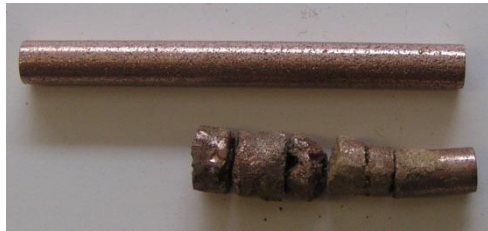
Figure 3.22: CuFe Taylor nail sample. Top: an original sample with a size of 6 mm diameter and a length of 60 mm. Bottom: fragments of the Taylor nail (3121) after an impact with a velocity of 217 m/s.
