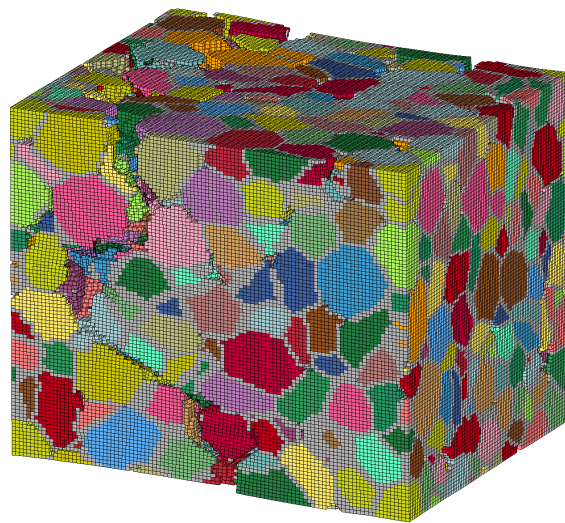
Figure 6.4: Cracked specimen at an elongation \varepsilon = 0.15/\text{ms} .
