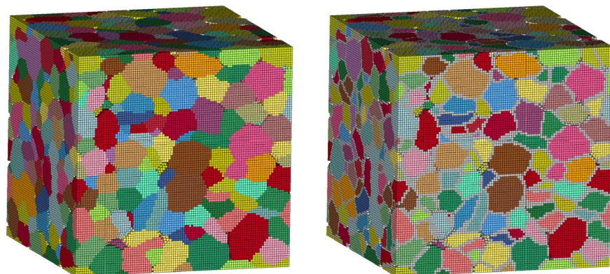
Figure 6.3: Introduction of grain boundary elements, left side: unmodified mesh with 958,363 elements, right side: mesh after introducing 276,979 boundary elements.
