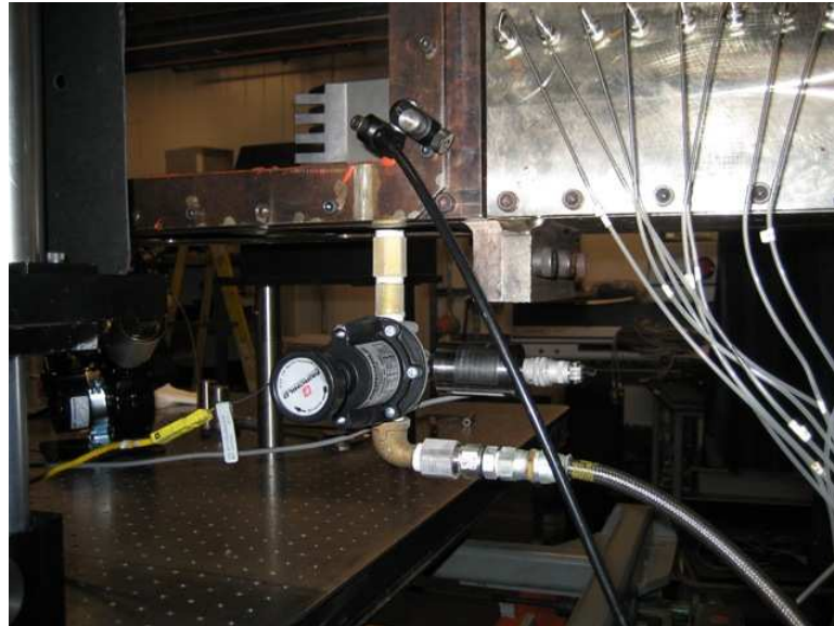
Fig. 4.6 Fairchild® model 10264 precision regulator.
