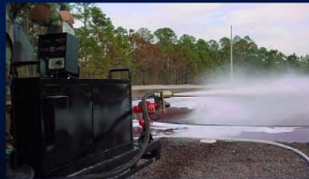
Apr 2004: Scale up - 100 gpm UHP Skid
