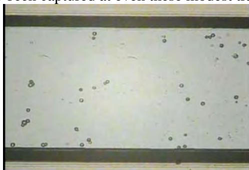
Figure 1: Cancer cells captured in a microchannel, 100µm deep and 1mm wide.
