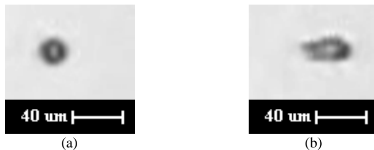
Figure 15. A captured BT20 cancer: (a) after incubation under no flow, and (b) after capture subject to a flow of 55\text{mm/s} .
