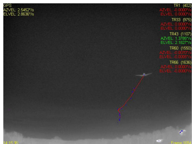
Figure 59: Video track of Piper aircraft using side by side L3 cameras at Pottstown Airport (Figure 28). Left hand side in the data logger GPS track, right hand side is the calculated track
