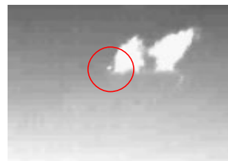
Figure 73: LWIR image of clouds using \mu bolometer. Red circle is an aircraft.
