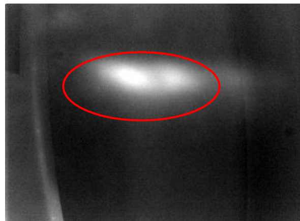
Figure 26: STD and average of the L-3 microbolometer. Note the red circle is a defect in the FPA.
