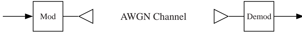
Figure 2.1: Basic digital communication system model showing transmitter modulation and receiver demodulation functions. An AWGN propagation channel is illustrated.
