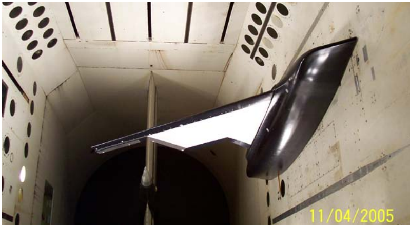
Figure 8. Batwing model in the NASA Langley TDT wind tunnel
