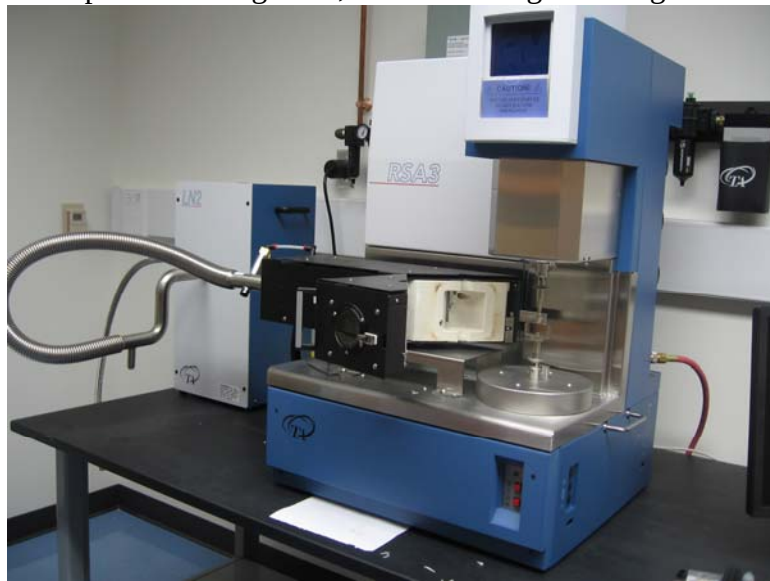
Figure 1. Illustration of DMA with liquid nitrogen cooling unit installed in the Polymer Research lab at Miami University.
