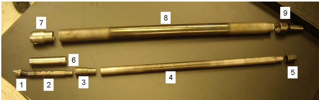
Figure D-1a. Modified Geoprobe® Groundwater Profiler - Components.
