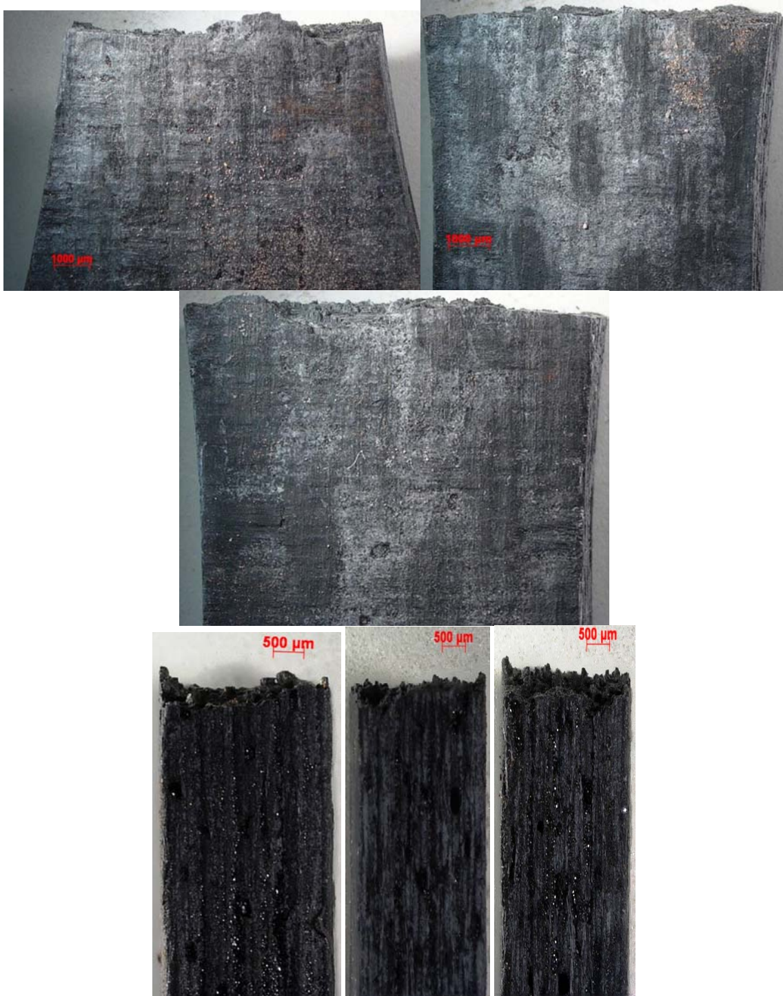
Figure 73. Fracture surface optical micrographs of composite C1 specimen fatigued in steam at 1300 °C with maximum fatigue stress \sigma_{\max} = 120 MPa
