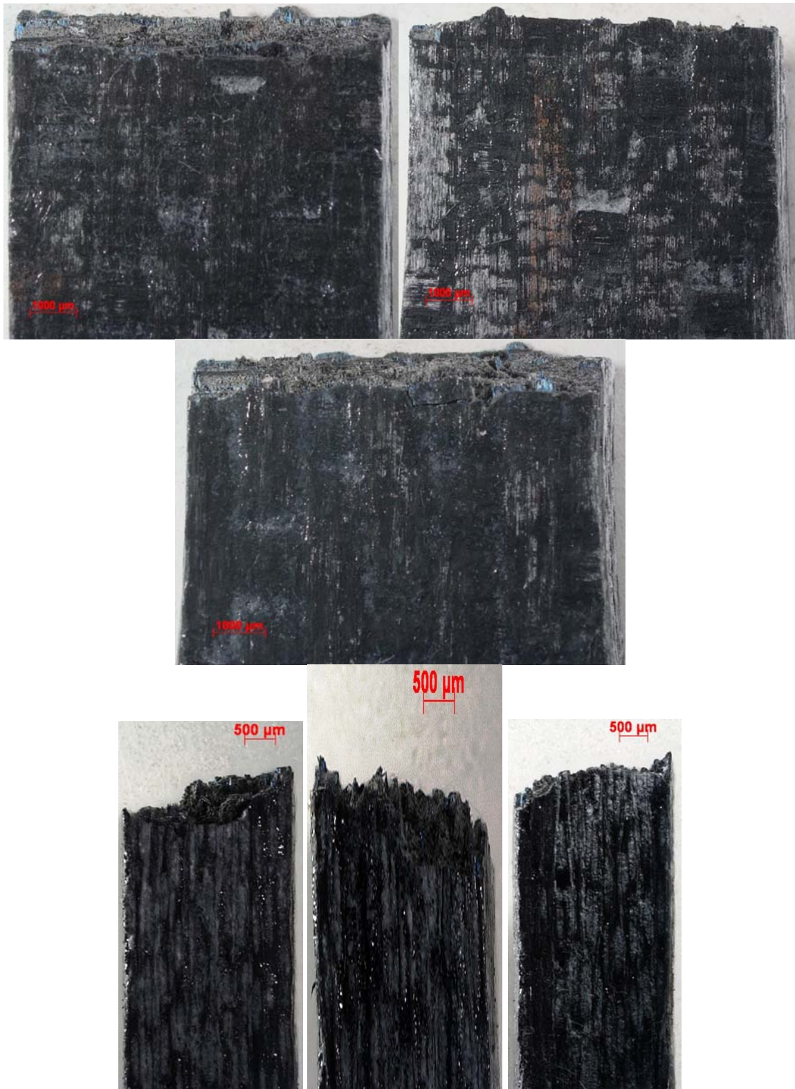
Figure 72. Fracture surface optical micrographs of composite C1 specimen fatigued in steam at 1300 °C with maximum fatigue stress \sigma_{\max} = 100 MPa
