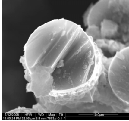
Figure 164. Fracture surface SEM micrograph of composite C3 specimen aged in steam for 8 hours at 815 °C and subjected to a monotonic tension test to failure.
