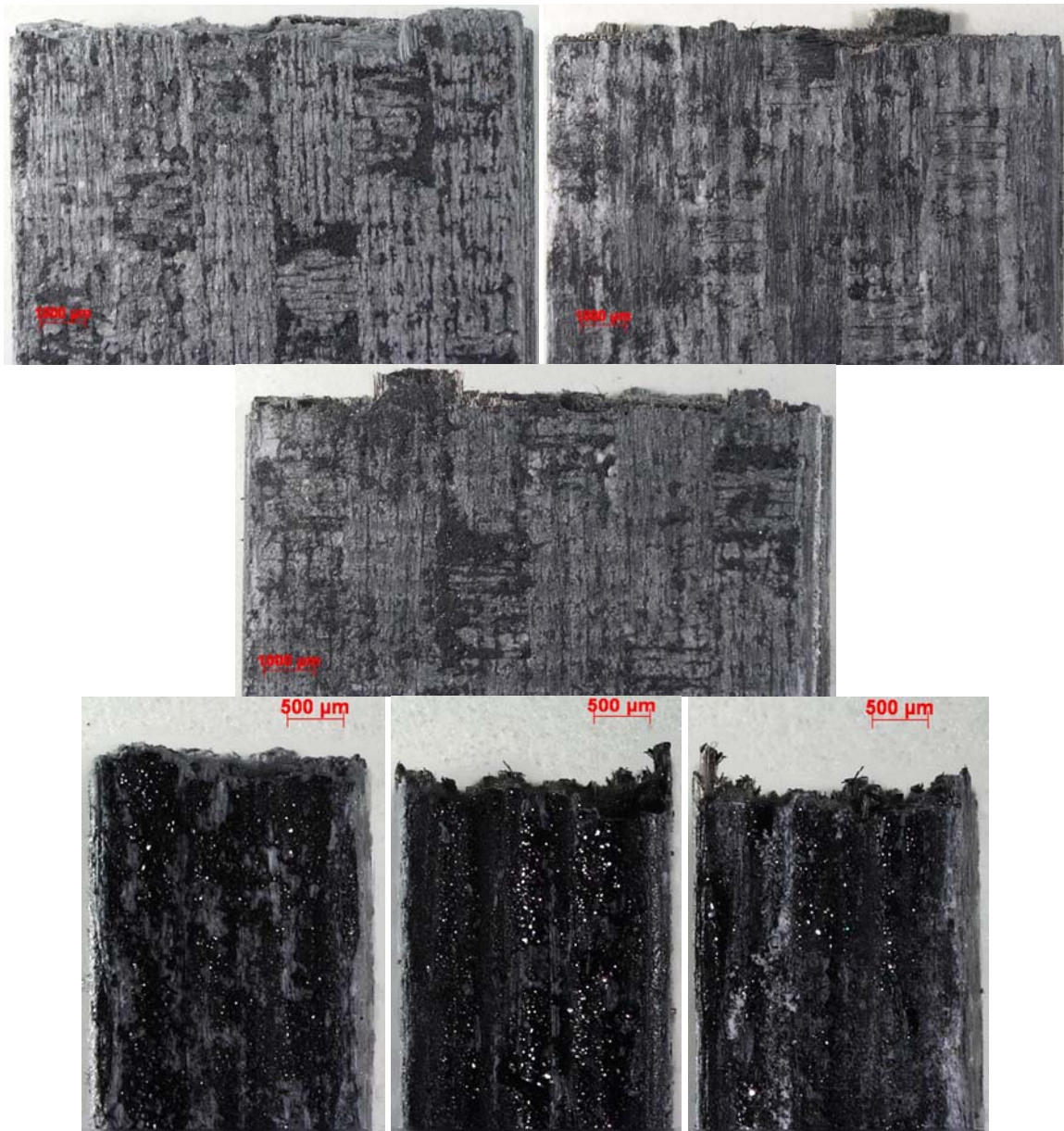
Figure 81. Fracture surface optical micrographs of composite C2 specimen fatigued in steam at 1300 °C with maximum fatigue stress \sigma_{\max} = 180 MPa
