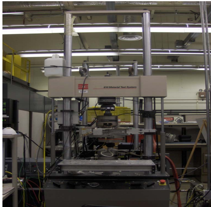
Figure 8. MTS System Corporation model 810 5 kip servo-hydraulic machine.
