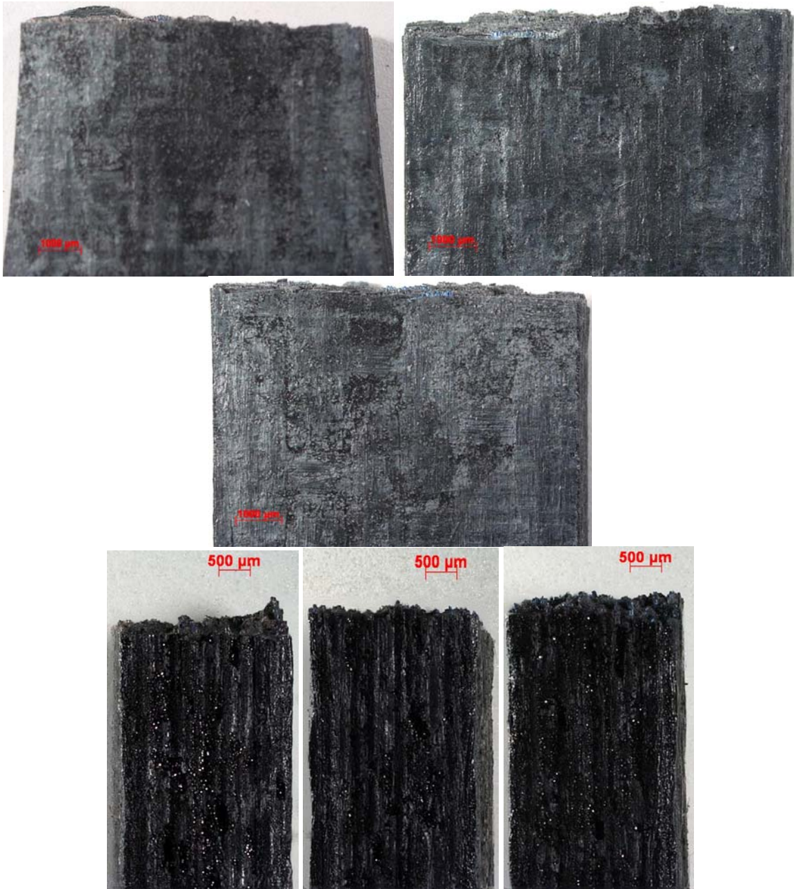
Figure 69. Fracture surface optical micrographs of composite C1 specimen fatigued in air at 1300 °C with maximum fatigue stress \sigma_{\max} = 100 MPa
