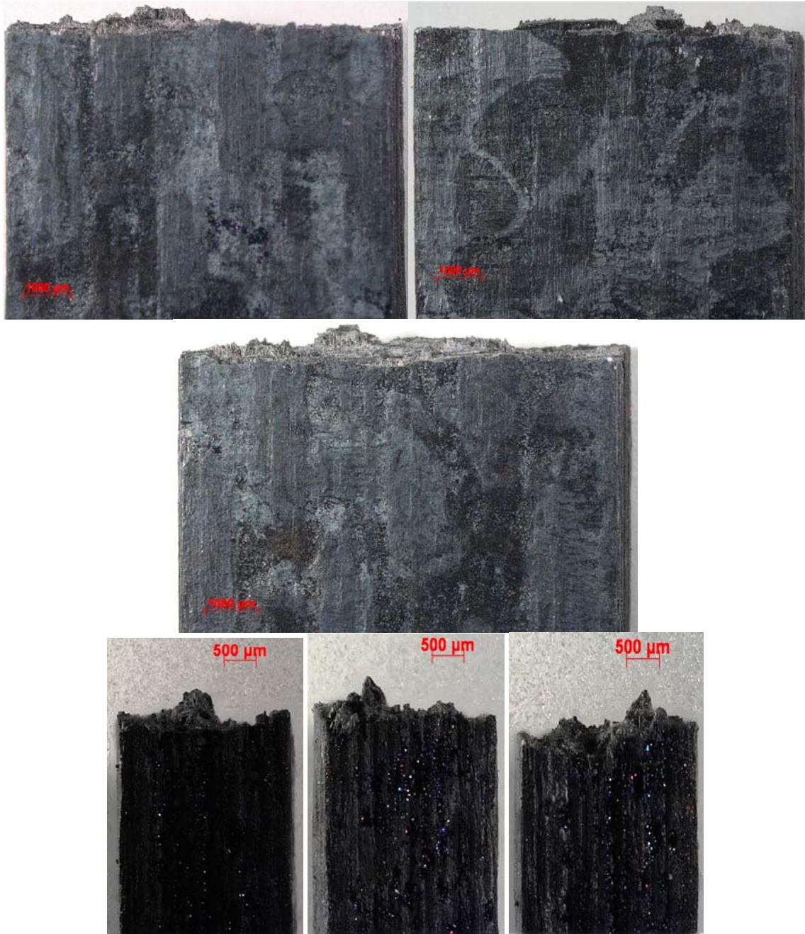
Figure 70. Fracture surface optical micrographs of composite C1 specimen fatigued in air at 1300 °C with maximum fatigue stress \sigma_{\max} = 120 MPa
