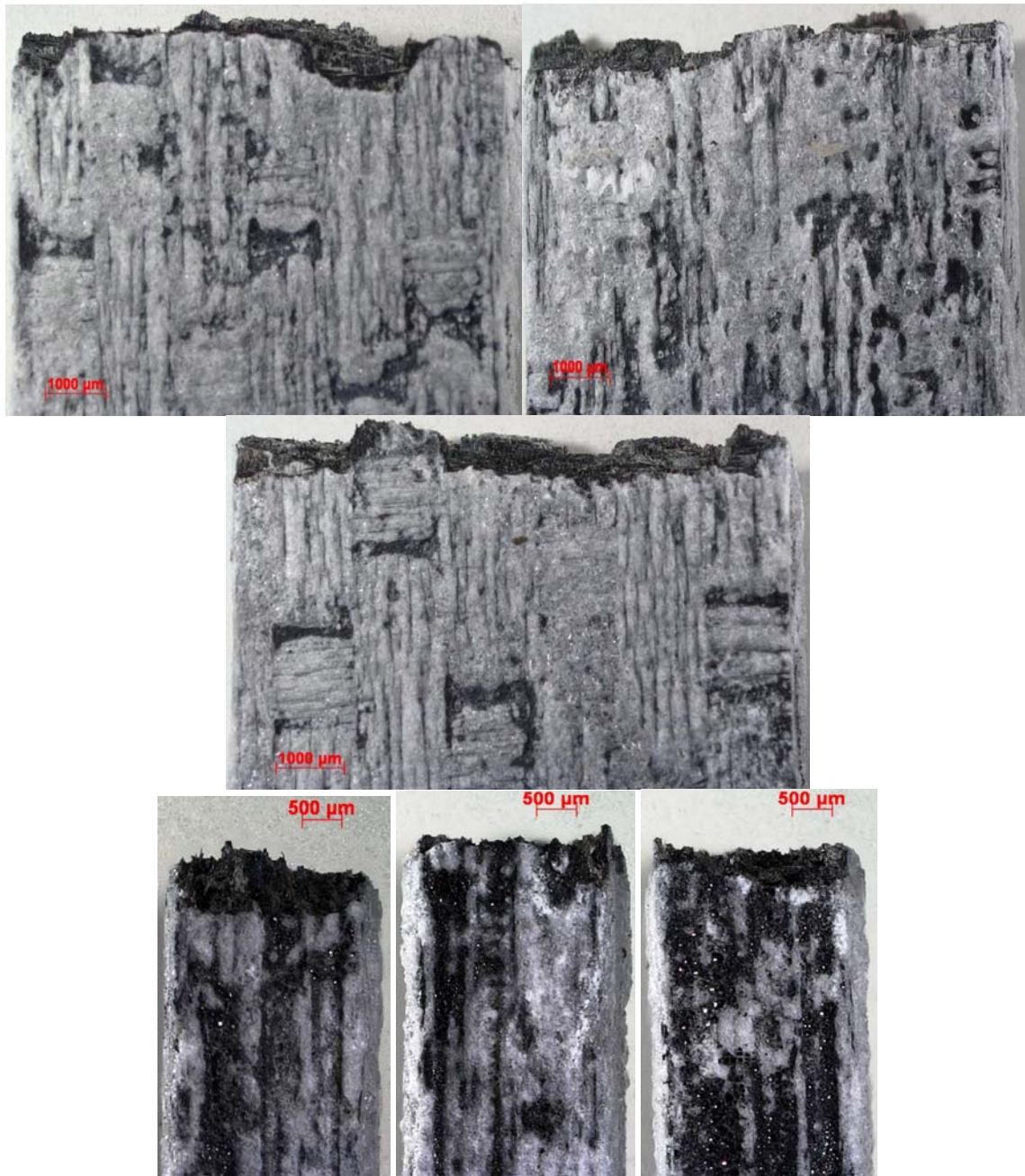
Figure 79. Fracture surface optical micrographs of composite C2 specimen fatigued in steam at 1300 °C with maximum fatigue stress \sigma_{\max} = 140 MPa
