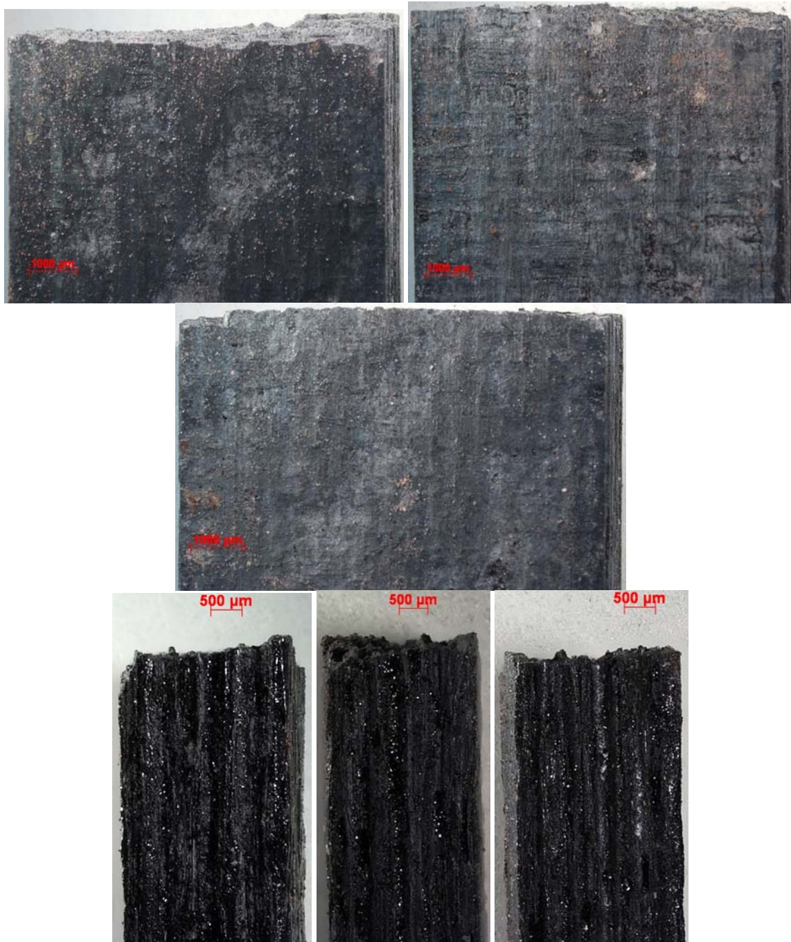
Figure 74. Fracture surface optical micrographs of composite C1 specimen fatigued in steam at 1300 °C with maximum fatigue stress \sigma_{\max} = 140 MPa
