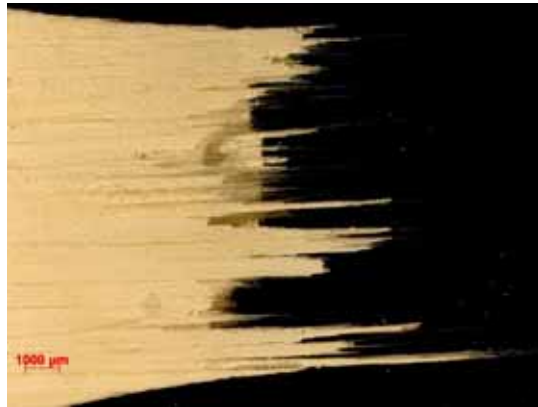
Figure B.91: Fracture surface of the N610/LaPO 4 /Al 2 O 3 specimen with 10ply 0°/90° uni-tape lay-up subjected to creep test at 120 MPa in steam at 1100 °C ( t_f = 0.03 h).
