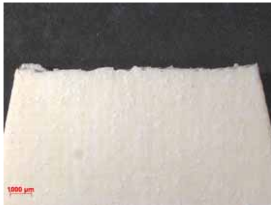
Figure B.10: Fracture surface of the N610/ \text{Al}_2\text{O}_3 - \text{LaPO}_4 specimen with 10ply 0^\circ/90^\circ uni-tape lay-up subjected tension to failure in laboratory air at 1100 °C.
