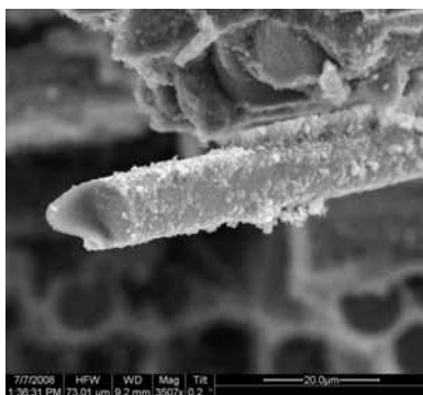
Figure A.396: Fracture surface of the N610/LaPO 4 /Al 2 O 3 -LaPO 4 -AlOCl specimen with 8ply HSW subjected to creep test at 32 MPa in air at 1100 °C ( t_f = 100h ).
