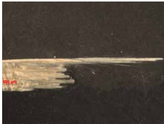
Figure B.61: Fracture surface of the N610/LaPO 4 /Al 2 O 3 specimen with 10ply 0°/90° uni-tape lay-up subjected to creep test at 85 MPa in air at 1100 °C ( t_f = 16.2 h).
