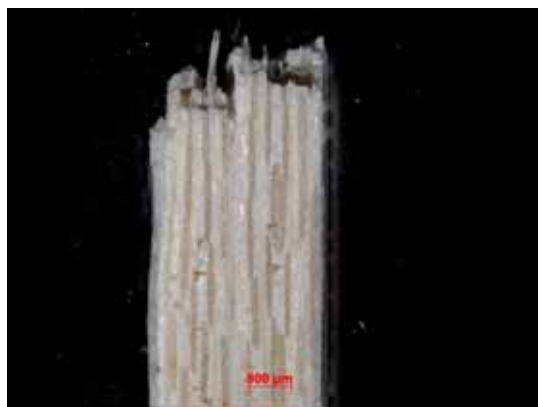
Figure B.233: Fracture surface of the N610/LaPO 4 /Al 2 O 3 -AlOCl specimen with 8ply HSW subjected subjected to creep test at 48 MPa in steam at 1100 °C ( t_f = 2.06 h).
