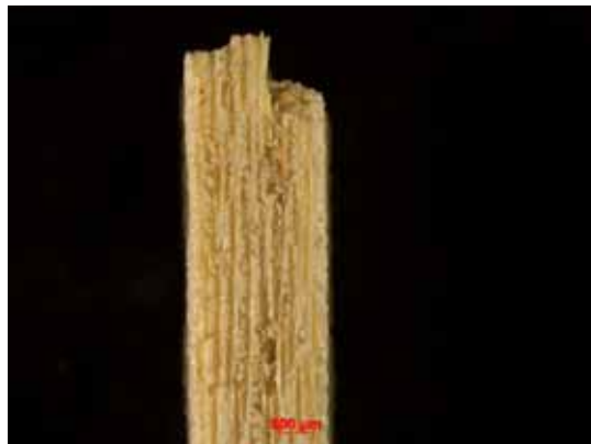
Figure B.181: Fracture surface of the N610/LaPO 4 /Al 2 O 3 specimen with 8ply HSW subjected subjected to creep test at 30 MPa in steam at 1100 °C ( t_f = 16.1 h).
