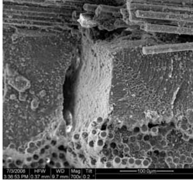
Figure A.157: Fracture surface of the N610/LaPO 4 /Al 2 O 3 specimen with 8ply HSW subjected to creep test at 32 MPa in air at 1100 °C ( t_f = 100\text{h} ).
