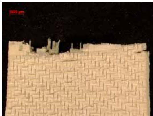
Figure B.118: Fracture surface of the N610/LaPO 4 /Al 2 O 3 specimen with 8ply HSW subjected subjected to creep test at 32 MPa in steam at 1100 °C ( t_f = 51.9 h).
