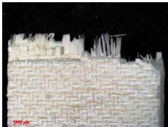
Figure B.139: Fracture surface of the N610/LaPO 4 /Al 2 O 3 specimen with 8ply HSW subjected subjected to creep test at 64 MPa in steam at 1100 °C ( t_f = 2.38 h).
