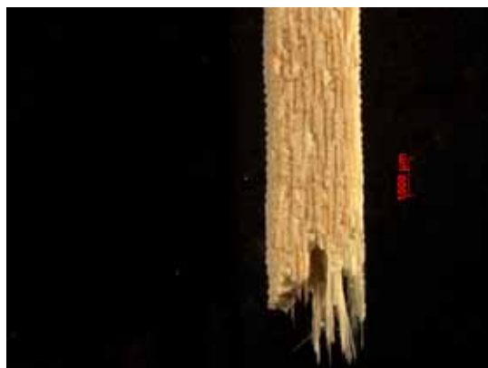
Figure B.103: Fracture surface of the N610/LaPO 4 /Al 2 O 3 specimen with 8ply HSW subjected tension to failure in laboratory air at 1100 °C.
