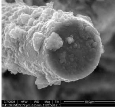
Figure A.420: Fracture surface of the N610/LaPO 4 /Al 2 O 3 -LaPO 4 -AlOCl specimen with 8ply HSW subjected to creep test at 32 MPa in steam at 1100 °C ( t_f = 3.47\text{h} ).
