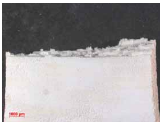
Figure B.215: Fracture surface of the N610/LaPO 4 /Al 2 O 3 -AlOCl specimen with 8ply HSW subjected subjected to creep test at 32 MPa in air at 1100 °C ( t_f > 100 h).
