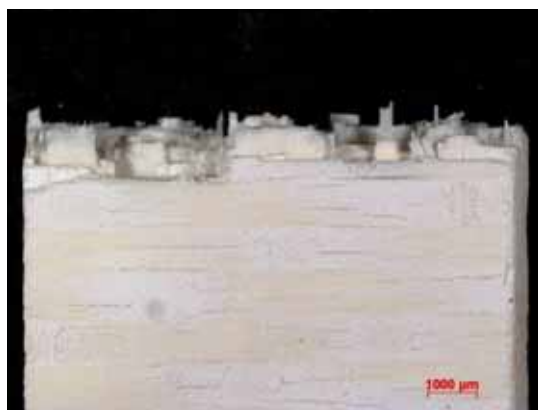
Figure B.232: Fracture surface of the N610/LaPO 4 /Al 2 O 3 -AlOCl specimen with 8ply HSW subjected subjected to creep test at 48 MPa in steam at 1100 °C ( t_f = 2.06 h).
