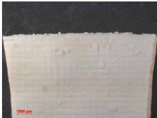
Figure B.5: Fracture surface of the N610/ \text{Al}_2\text{O}_3 - \text{LaPO}_4 specimen with 10ply 0^\circ/90^\circ uni-tape lay-up subjected tension to failure in laboratory air at 1100^\circ\text{C} .
