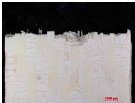
Figure B.231: Fracture surface of the N610/LaPO 4 /Al 2 O 3 -AlOCl specimen with 8ply HSW subjected subjected to creep test at 48 MPa in steam at 1100 °C ( t_f = 2.06 h).
