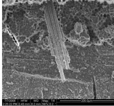
Figure A.409: Fracture surface of the N610/LaPO 4 /Al 2 O 3 -LaPO 4 -AlOCl specimen with 8ply HSW subjected to creep test at 32 MPa in steam at 1100 °C ( t_f = 3.47\text{h} ).
