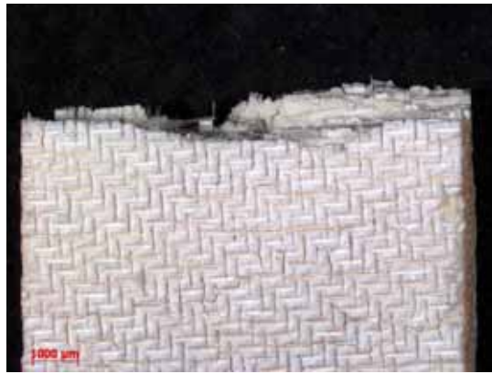
Figure B.147: Fracture surface of the N610/LaPO 4 /Al 2 O 3 specimen with 8ply HSW subjected subjected to creep test at 72 MPa in air at 1100 °C ( t_f > 100 h).
