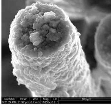
Figure A.234: Fracture surface of the N610/LaPO 4 /Al 2 O 3 specimen with 8ply HSW subjected to creep test at 72 MPa in steam at 1100 °C ( t_f = 2.24\text{h} ).
