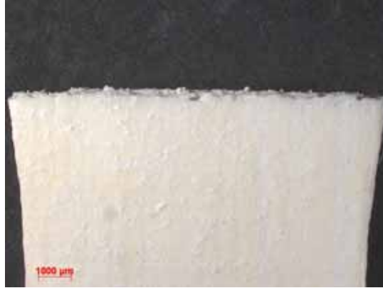
Figure B.6: Fracture surface of the N610/ \text{Al}_2\text{O}_3 - \text{LaPO}_4 specimen with 10ply 0^\circ/90^\circ uni-tape lay-up subjected tension to failure in laboratory air at 1100 °C.
