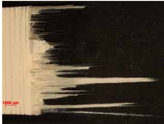
Figure B.75: Fracture surface of the N610/LaPO 4 /Al 2 O 3 specimen with 10ply 0°/90° uni-tape lay-up subjected to creep test at 110 MPa in steam at 1100 °C ( t_f = 0.35 h).
