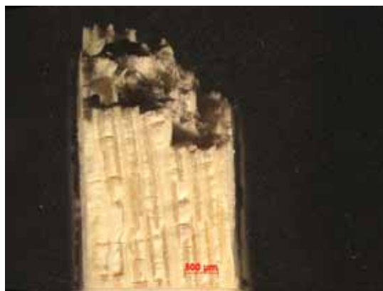
Figure B.229: Fracture surface of the N610/LaPO 4 /Al 2 O 3 -AlOCl specimen with 8ply HSW subjected subjected to creep test at 32 MPa in steam at 1100 °C ( t_f = 3.47 h).
