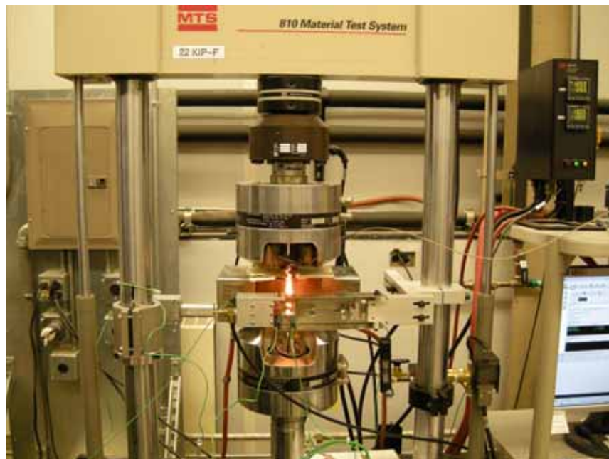
Figure 4.3: Close-up view of the MTS machine and the extensometer.
