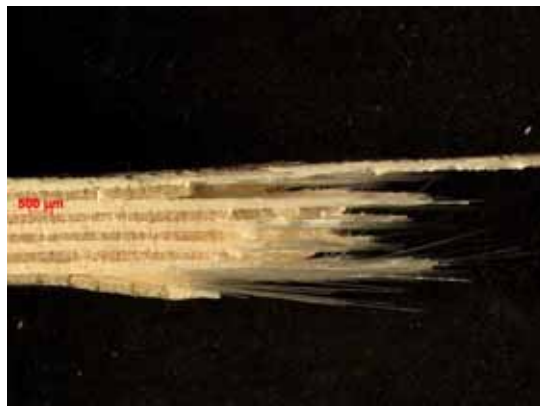
Figure B.55: Fracture surface of the N610/LaPO 4 /Al 2 O 3 specimen with 10ply 0°/90° uni-tape lay-up subjected tension to failure in laboratory air at 1100 °C.
