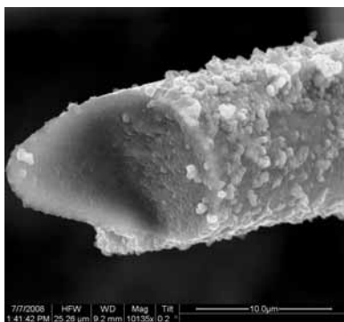
Figure A.398: Fracture surface of the N610/LaPO 4 /Al 2 O 3 -LaPO 4 -AlOCl specimen with 8ply HSW subjected to creep test at 32 MPa in air at 1100 °C ( t_f = 100h ).
