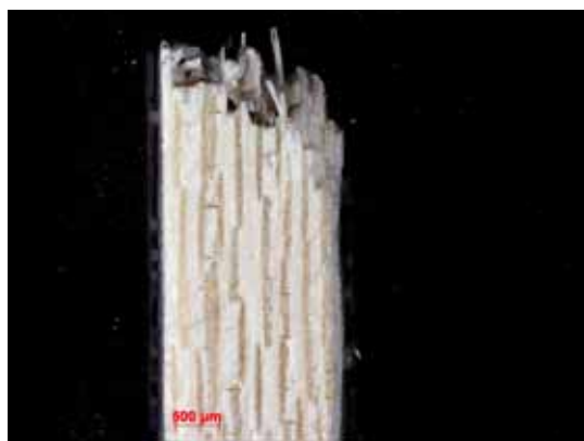
Figure B.234: Fracture surface of the N610/LaPO 4 /Al 2 O 3 -AlOCl specimen with 8ply HSW subjected subjected to creep test at 48 MPa in steam at 1100 °C ( t_f = 2.06 h).
