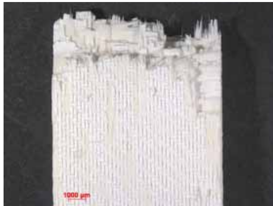
Figure B.153: Fracture surface of the N610/LaPO 4 /Al 2 O 3 specimen with 8ply HSW subjected subjected to creep test at 72 MPa in steam at 1100 °C ( t_f = 2.24 h).
