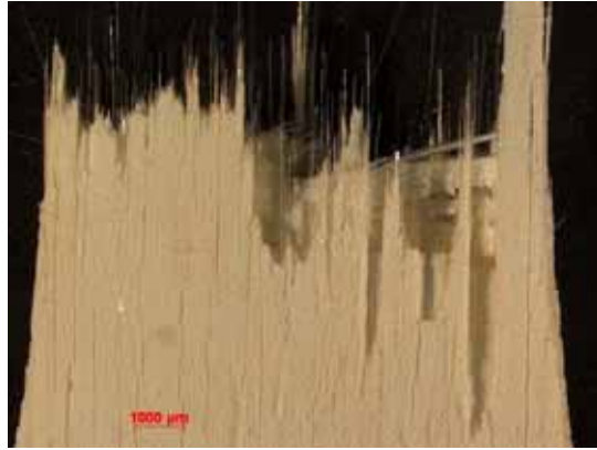
Figure B.53: Fracture surface of the N610/LaPO 4 /Al 2 O 3 specimen with 10ply 0°/90° uni-tape lay-up subjected tension to failure in laboratory air at 1100 °C.
