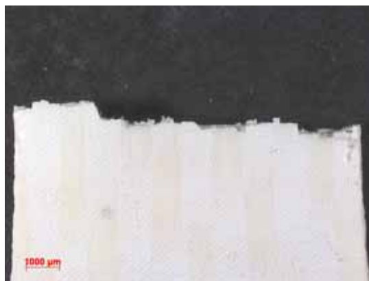
Figure B.214: Fracture surface of the N610/LaPO 4 /Al 2 O 3 -AlOCl specimen with 8ply HSW subjected subjected to creep test at 32 MPa in air at 1100 °C ( t_f > 100 h).
