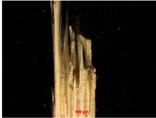
Figure B.74: Fracture surface of the N610/LaPO 4 /Al 2 O 3 specimen with 10ply 0°/90° uni-tape lay-up subjected to creep test at 110 MPa in steam at 1100 °C ( t_f = 0.35 h).
