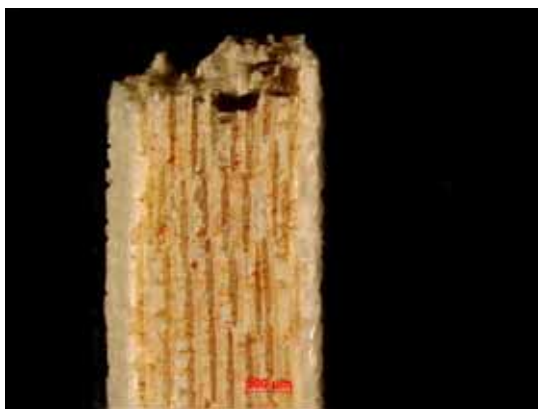
Figure B.191: Fracture surface of the N610/LaPO 4 /Al 2 O 3 specimen with 8ply HSW subjected subjected to creep test at 40.5 MPa in air at 1100 °C ( t_f = 3.34 h).
