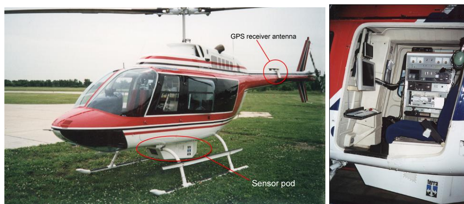
Figure 2-1 Helicopter-mounted Lidar and Orthophoto Sensor Equipment
