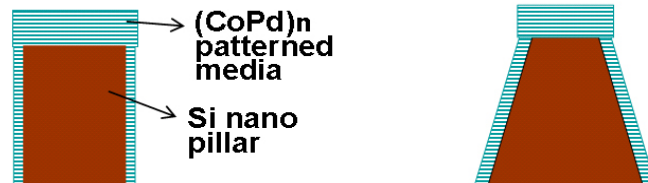
Fig. 5. Schematic illustration of undesirable sidewall deposition of magnetic recording media for vertical or positively tapered nano-pillar structure.
