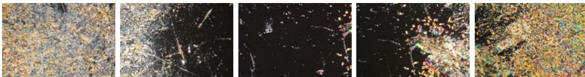
Figure III. Polarized optical microscopy conducted in a lateral sweep across the center of a 5CB droplet that is on a thin film of side-on SGLCP. The center of this droplet displays homeotropic anchoring.
