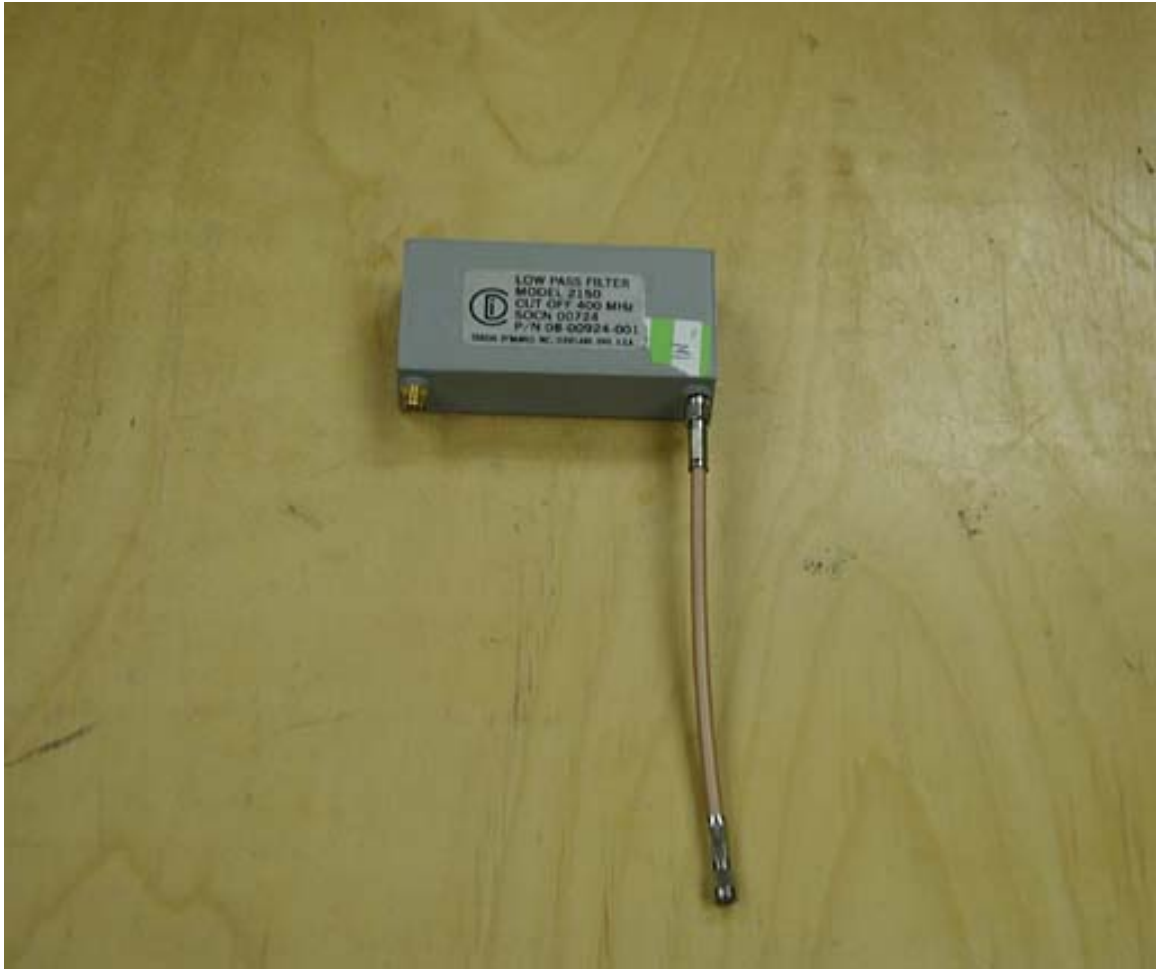
Figure 65. Functional Block I: low-pass filter.
