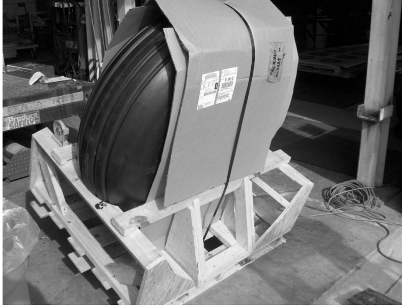
Figure 3a. Tip Test – on side of cradle.
