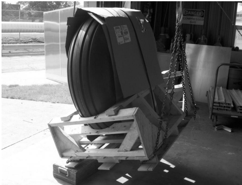
Figure 10. Rotational Corner Drop Test –18” height.
