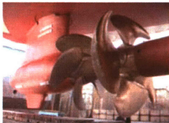
Fig. 2. High-speed ferry “Hamanasu” with hybrid CRP-POD propulsion system
