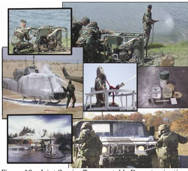
Figure 10 - Joint Service Transportable Decontamination System – Small Scale
