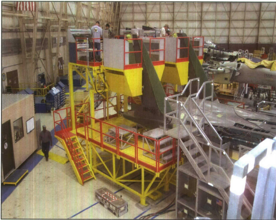
Warner Robins Air Logistics Center performs the F-15 programmed depot maintenance. By using Lean methodologies and the tools in the Air Force Smart Operations for the 21 st Century toolbox, the center has streamlined the process to return the F-15 Eagles back to the warfighter on time, on cost, and at improved quality. One of the AFSO21 events culminated in the development of the tail stands shown in this picture. These stands allow workers on either side of the tail to raise or lower their platform to better accommodate their body height. Mechanics also have their tools on hand and avoid constantly going up and down the steps to retrieve tools needed to perform each task. The F-15 PDM line, the F-15 avionics shop and the F-15 wing shop have all been bronze recipients of the Shingo Award.
