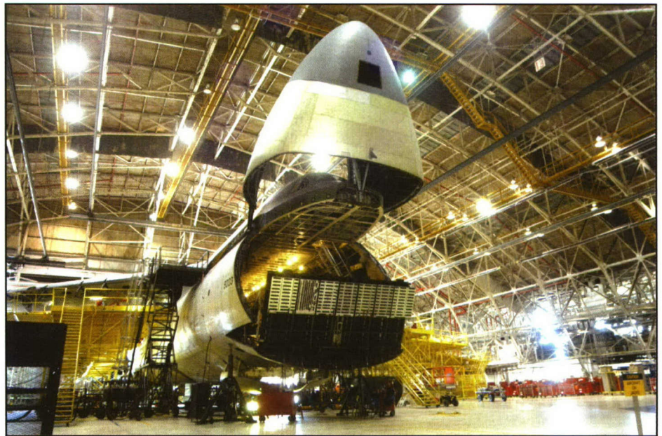
C-5 Programmed Depot Maintenance work is carried out at the Warner Robins Air Logistics Center. When this aircraft, the largest cargo jet in the US Air Force fleet, first arrived at the center it took longer than 300 days to complete the PDM. Through Air Force Smart Operations for the 21 st Century initiatives, the PDM process is now averaging less than 170 days. Because of the continuous process improvement initiatives put in place by the C-5 PDM program, the center has received two gold Shingo awards—first in 2005 and again in 2006—as well as the Franz Edelman Award for Achievement in Operations Research in 2006.
