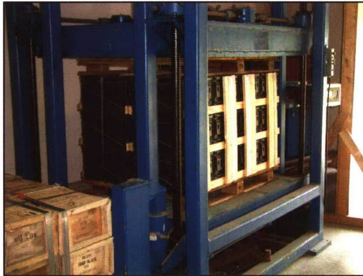
Photo 7. Test Unit #1 in the Stacking Test.
