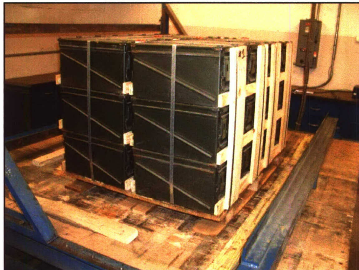
Photo 8. Test Unit #1 During Repetitive Shock Testing.
