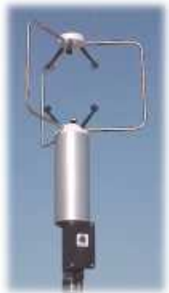
A 3-D (u,v,w) sonic anemometer
