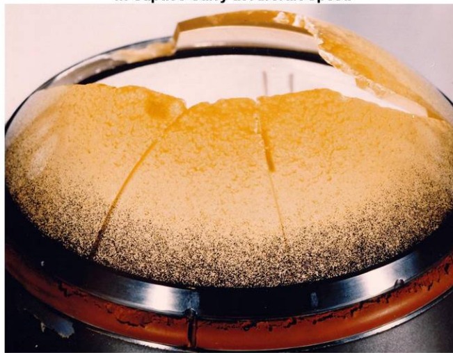
Figure 162. Zinc sulfide Maverick missile dome fractured due to rain impact.
