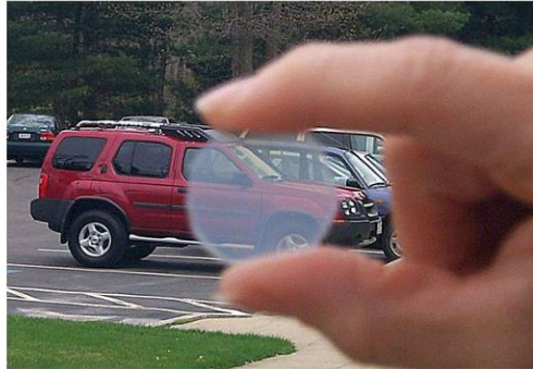
Cera Nova alumina has modest visible transparency, but good infrared transparency
