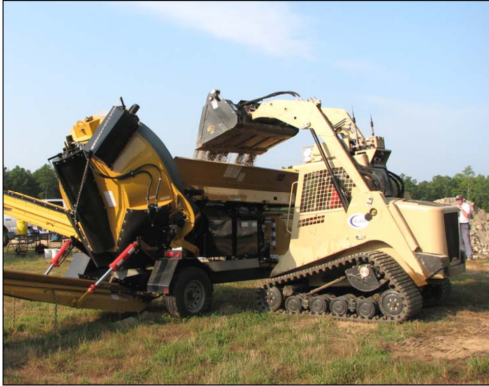
Figure 27: ASV SR-80 Loader in Operation
