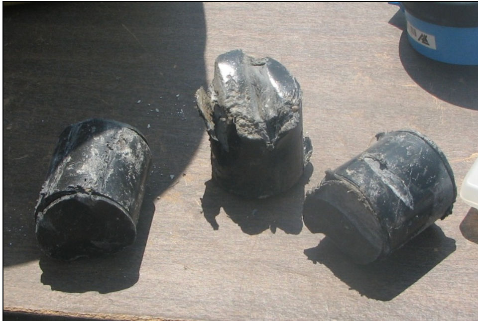
Figure 20: PVC Mine Simulants, 50 mm Setting
