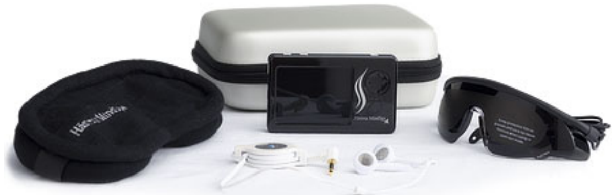
Figure 2. Prototype system for delivery of LED generated light flashes to the eyes through either a sleep mask (left side) or goggles (right side). The control unit is incorporated into an MP3 player shown in the center.
