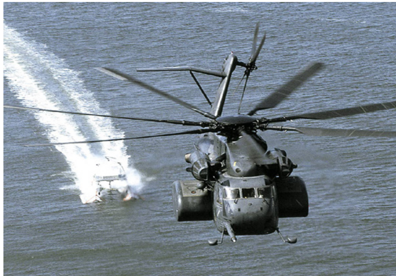
Figure 43: MH-53E Towing a Sonar Array Sled
