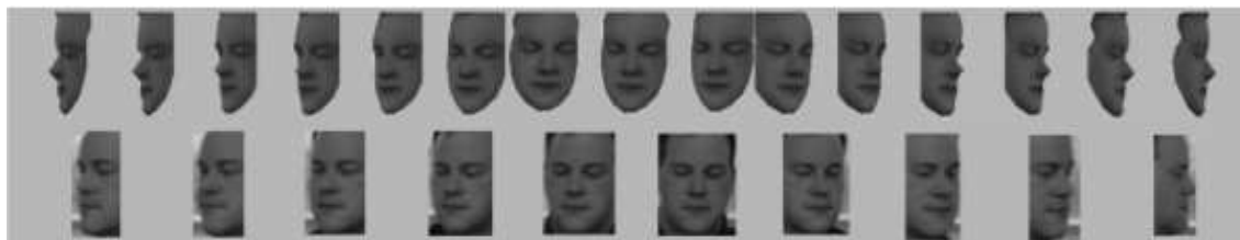
Figure 4.12. Face matching: the top row shows the 15 training images generated from the 3D model; the bottom row shows 10 test images of the subject captured from a CCD camera.
