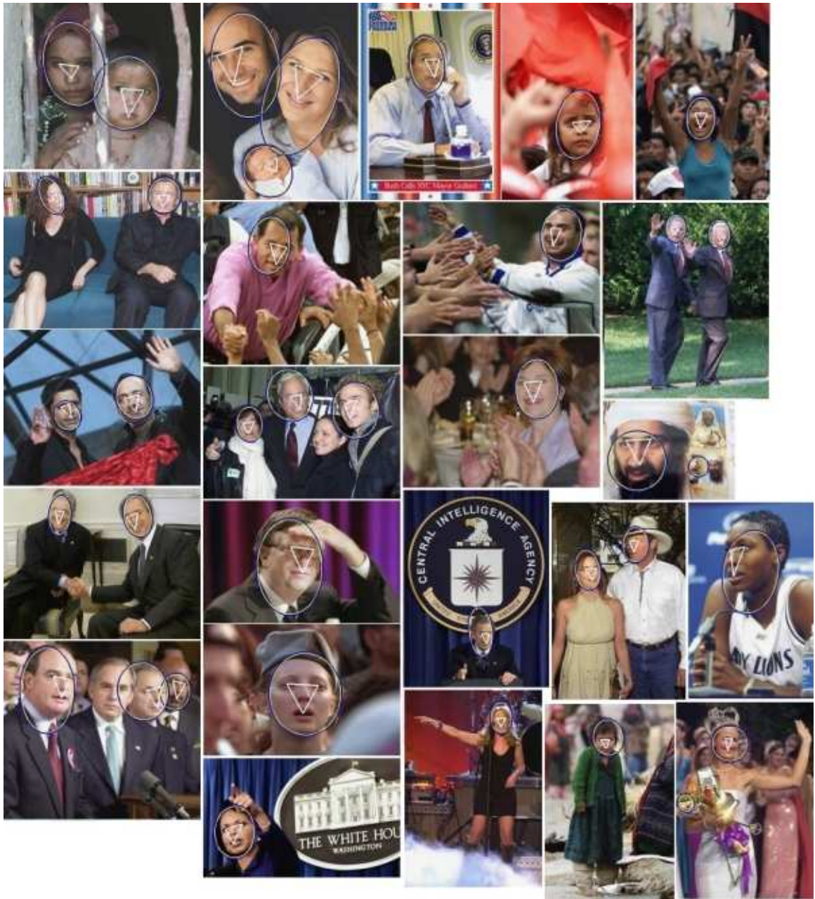
Figure 3.23. Face detection results on a subset of 24 news photos. The detected faces are overlaid on the color-compensated images. False negatives are due to extreme lighting conditions, shadows, and low image quality (i.e., high compression rate).
