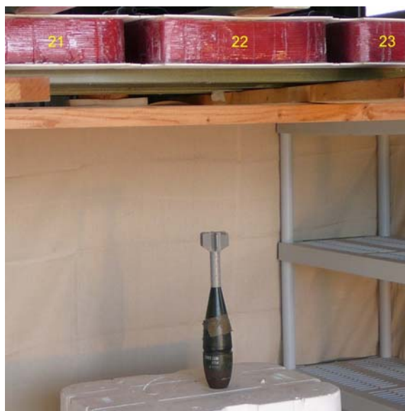
Figure 4 – 81-mm mortar placed under the TEM array. Sensors 21, 22, and 23 are visible.
