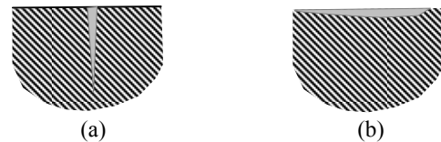
Figure.1 Types of damages: (a) Crack (b) Worn-out or corroded surface
