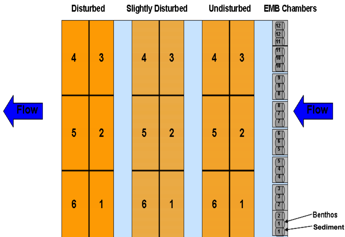
Figure 12. Schematic of the Experimental Design of Both the Embeddedness Chambers and the Treatment Areas. Two Numbers from Each Treatment Area Were Randomly Selected For Each Sampling Event. Four Embeddedness Chamber Numbers (both for benthos and sediment) Were Randomly Selected for Each of the Three Sampling Events.
