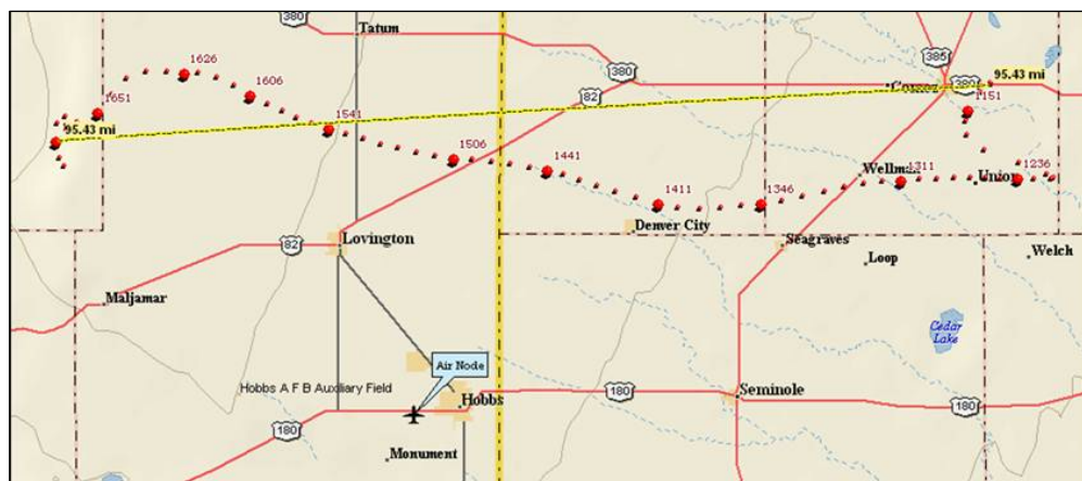
Fig. 32 — Flight path for the first UHF relay payload test, June 24 (UHF Flight 1). Two ground nodes were located near the launch site at Terry County Airport, and a third was flown out to Hobbs Airport, New Mexico.
