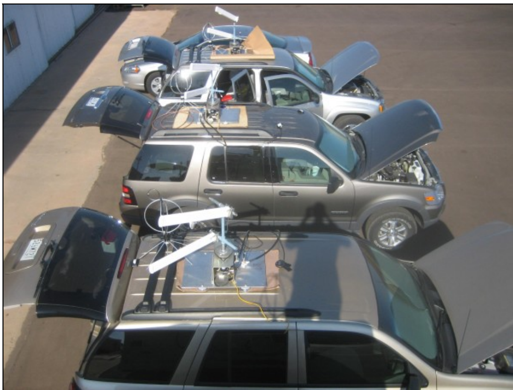
Fig. 4 — Antenna controllers on top of the sport utility vehicles. Each vehicle has two directional antennas, one for transmit and one for receive.
