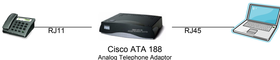
Fig. 31 — Setup diagram for VoIP testing.
