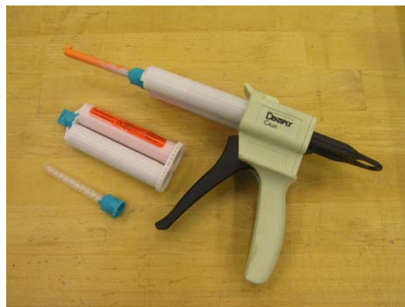
Figure C-3: Photo of an application gun with Aquasil Ultra cartridge and mixing tube
