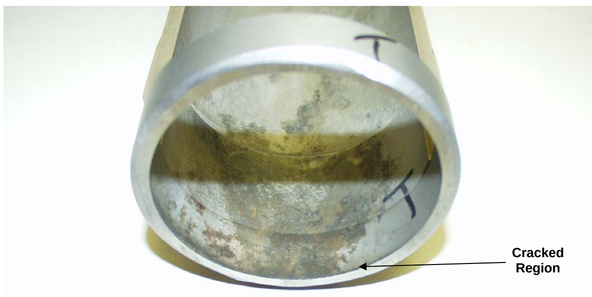
Figure F-16: Section of Shank PT0099 with Noncritical Fatigue Cracks (Forward of Lateral Damper Region)
