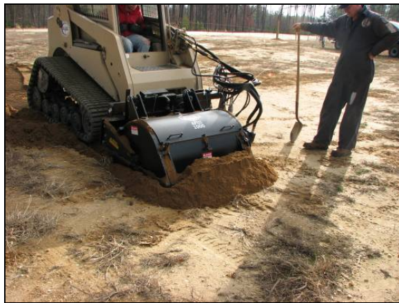
Figure 43: Dirt Buildup in front of Planer
