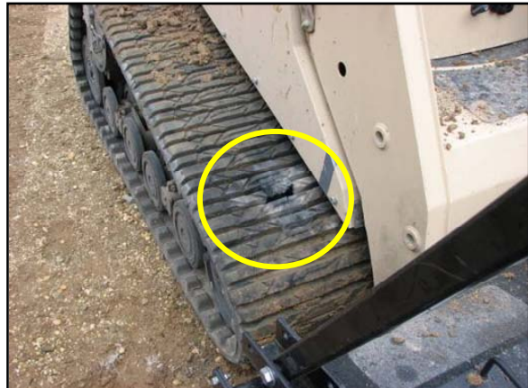
Figure 67: Damage to Track Exterior, Mine C
