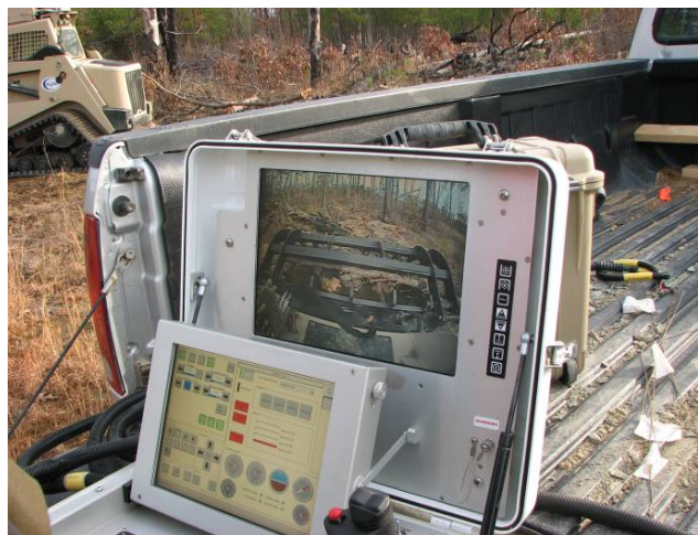
Figure 35: Remotely Controlling Nemesis with Operator Control Unit
