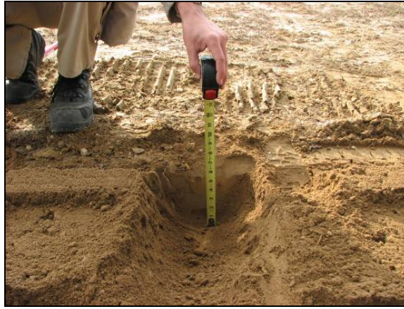
Figure 41: Penetration Depth of Planer in Manual Operations
