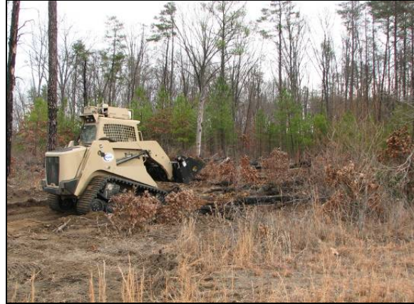
Figure 37: Scooping Small Debris with the 4-in-1 Bucket
