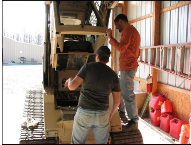
Figure 21: Cab Raised for Maintenance Inspection
