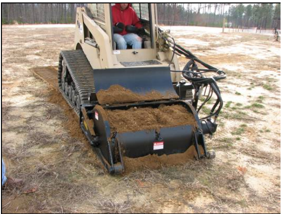
Figure 42: Dirt Buildup Inside Planer
