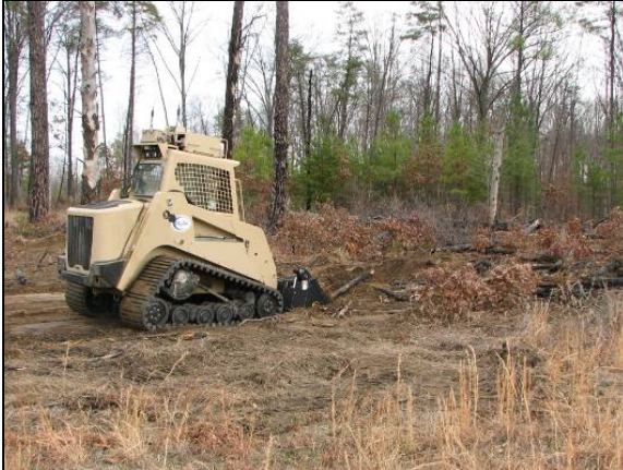
Figure 36: Scooping Small Debris with the 4-in-1 Bucket
