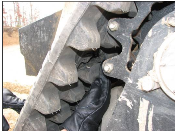
Figure 65: Damage to Track Interior, Mine A
