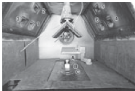
Figure 1. Photograph of EB-PVD chamber
