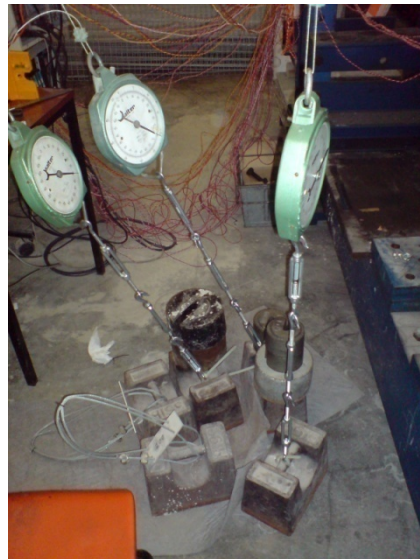
Figure 6-16. Scales in line with cable, turnbuckles and weights.
