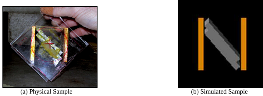
Figure 6. Composite iron-copper tomographic sample used for validation of the MLEM reconstruction algorithm. The sample is made up of copper (outer, vertical bars) and iron (inner, diagonal bars) arranged like the letter N. Each bar measures 6mm in thickness, 60mm in height and 24mm in depth. The sample was simulated in GEANT 4 as shown in (b). (Figure from [12]).
