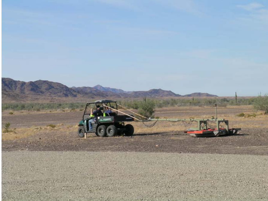
Figure 1. Demonstrator's system, EM61 MKII/towed array.
