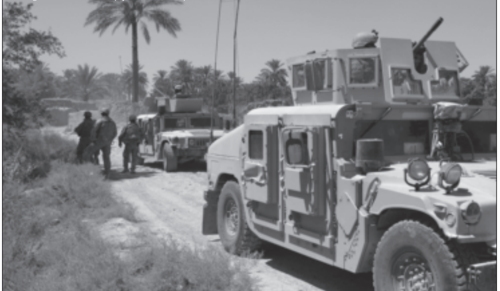
ARDEC designed and produced the first generation O-GPK to better protect vehicle gunners. The O-GPK system includes transparent armor windows and rearview mirrors that provide 100 percent visibility for the gunner. (U.S. Army photo courtesy of ARDEC.)
