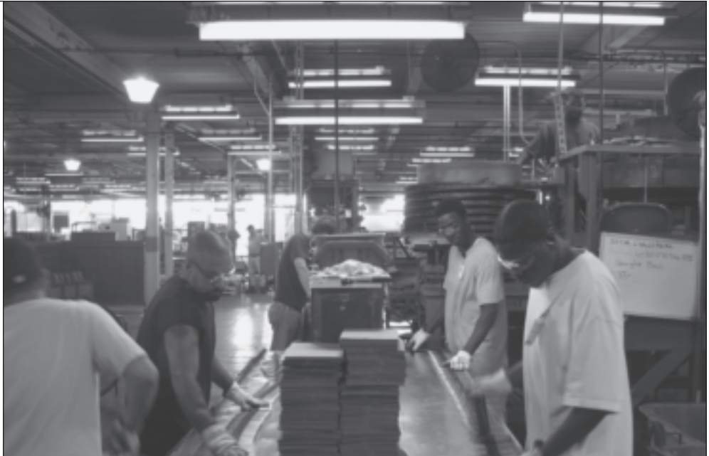
LCAAP workers ensure all .50-caliber ammunition belts are "stretch/flex" tested and visually inspected before being packed in M241 ammo cans for shipment or storage. (U.S. Army photo courtesy of LCAAP)
