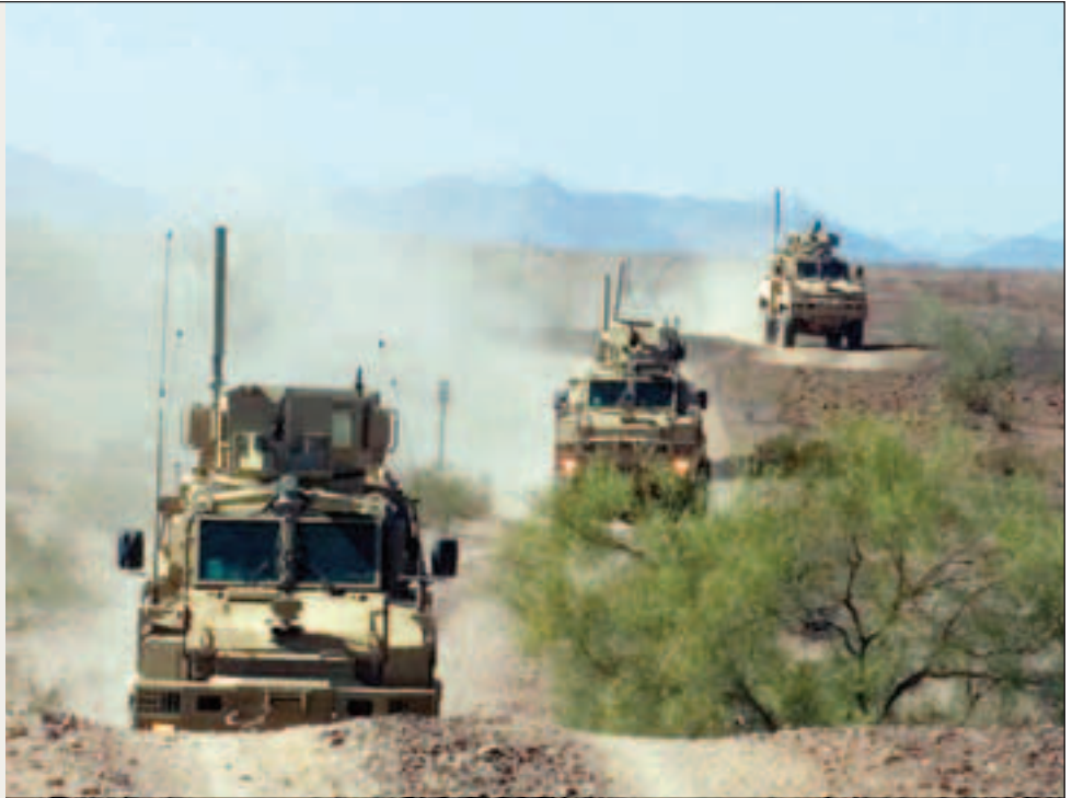
A variant of the MRAP vehicle undergoes grueling cross-country road evaluation during operational testing conducted by Soldiers and ATEC personnel at White Sands Missile Range, NM. (Photo courtesy of U.S. Army Operational Test Command.)
