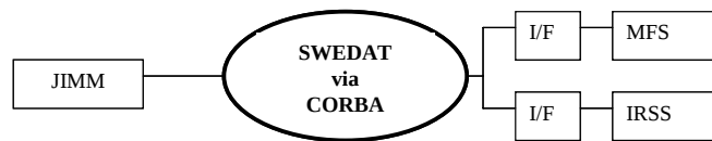
Figure 7 – Notional Exercise using JIMM and SMILE with Manned Flight and the IR stimulator.
