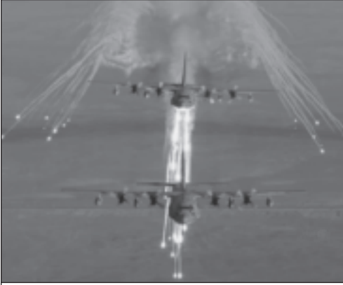
USAF transport planes preemptively fire countermeasure flares during take-off and landing, as those are the times when they are most vulnerable to shoulder-fired IR missiles. (DOD photo by SA Julianne Showalter.)
