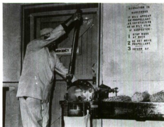
FIG. 4. Stick propellant being cut to suitable length for make-up of charges.
