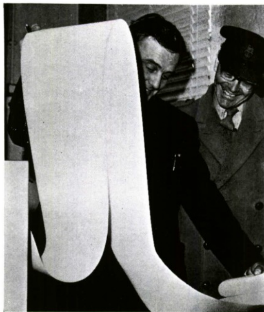
FIG. 10. Instrumentation Officer reading piezoelectric pressure and pressure difference from Ampex Tape Recorder.
