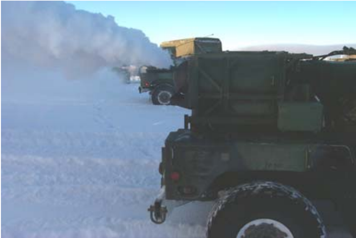
Figure 2. Close-up of an M157A2 fog oil aerosol generator during operation.
