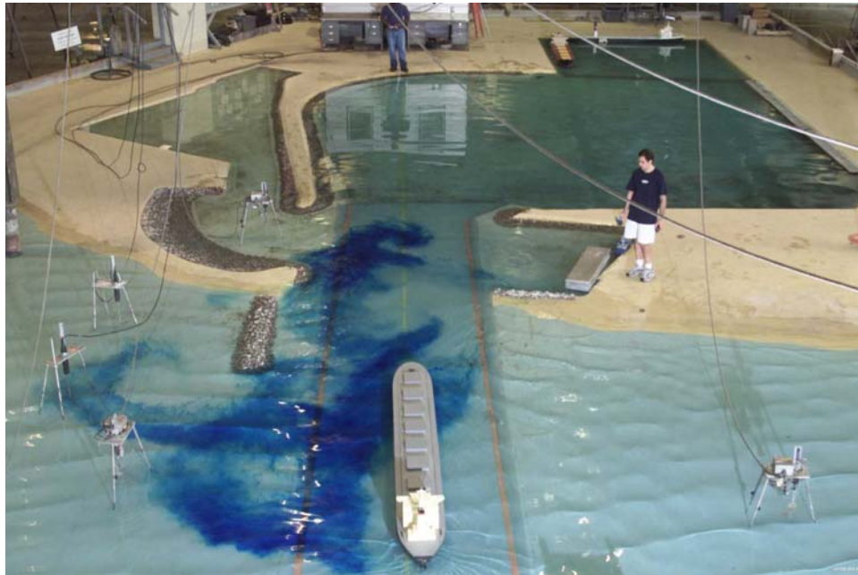
(c) Current flow is mainly to west, curling around jetty.
