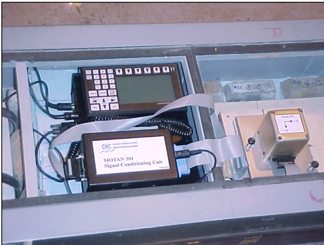
Figure 12. Typical installation for MOTAN motion analysis system.
