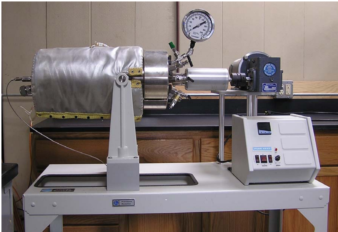
Figure 7. Parr reactor vessel used to mimic conditions inside hydrolyzer. Test material was kept at a set temperature within the heat-jacketed vessel on the left, while being constantly stirred by the motor on the right.
