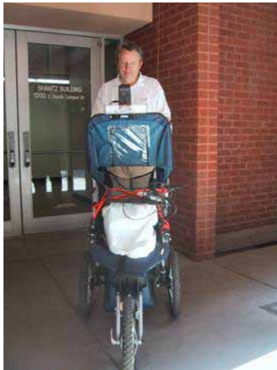
Figure 3. Receiver equipment on jogging stroller.
