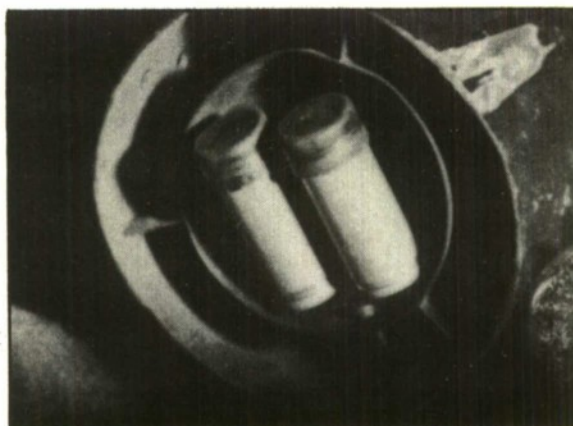
IGNITERS IN POSITION
