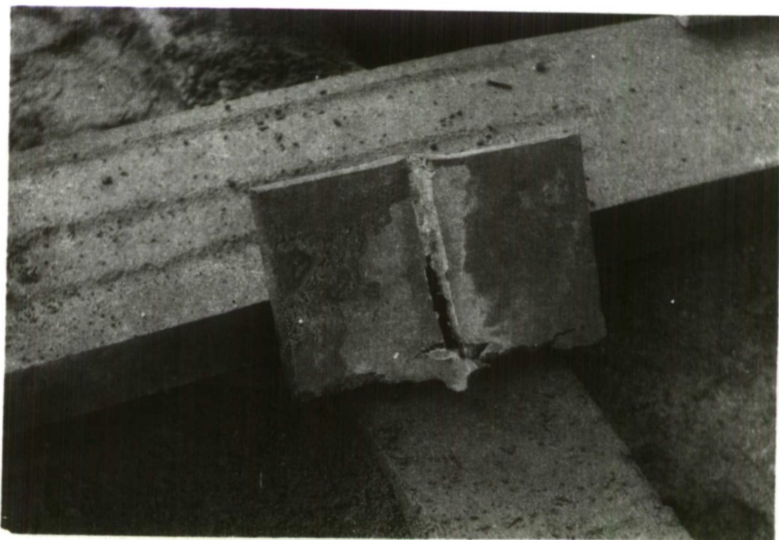
Photo No. 11. The 1\frac{1}{2} " plate after being cut by 8-oz. cartridge of P.E.
