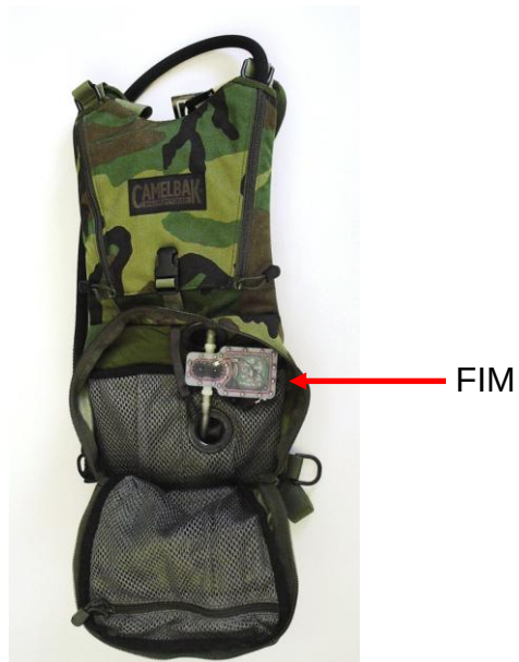
Figure 2. Modified Camelbak™ hydration system with Fluid Intake Monitor (FIM) inserted into the front pocket of the carrier
