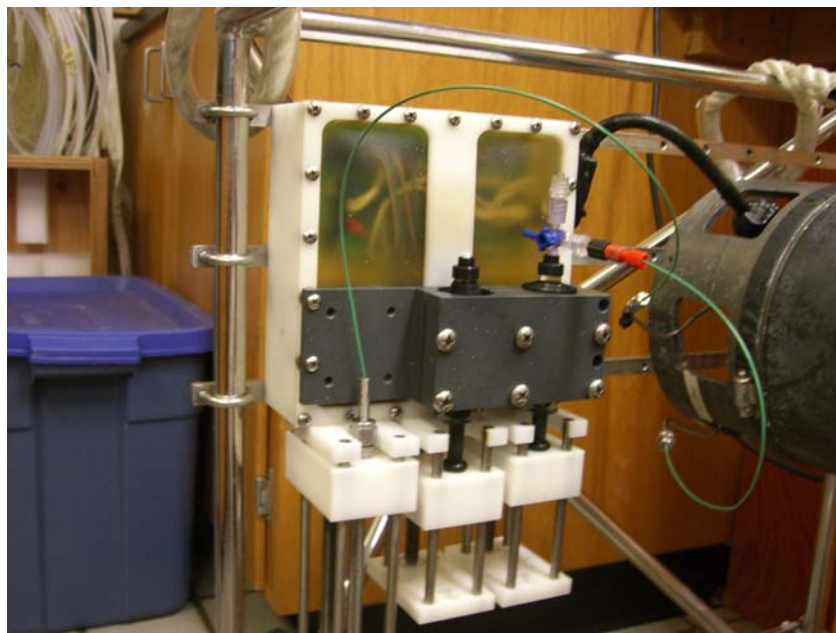
Figure 1. Photograph of positive displacement syringe pump system that provides constant flow sampling and the capability to add reagents to the sampling stream.
