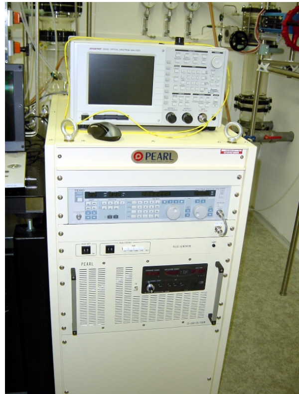
Photo 13. RF discharge source (details in text)
