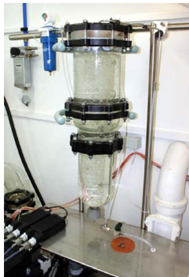
Photo 16. Glass tank for sodium thiosulphate solution or water for trap cleaning
