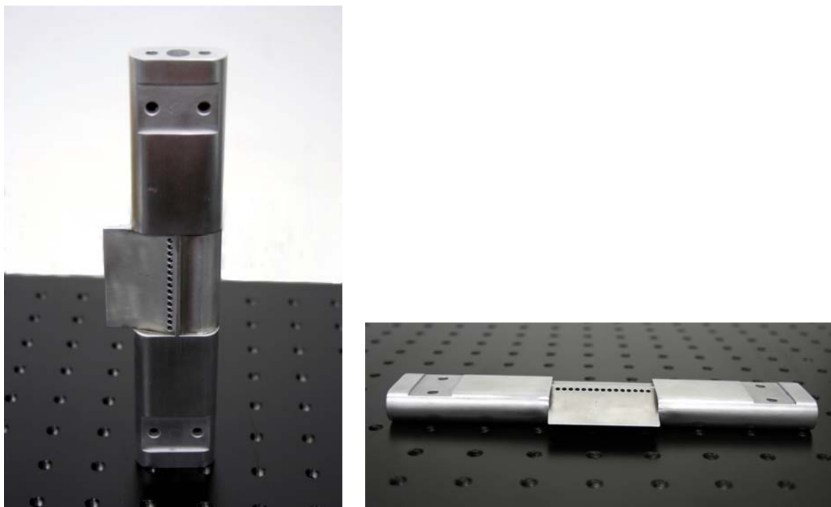
Photo 1. Iodine injector/supersonic nozzle (middle part of body)
